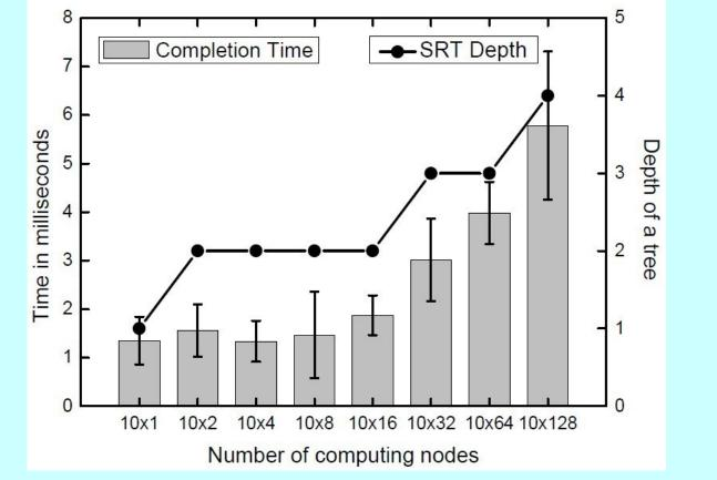
Latency is as low as 10 millisecond for query completion time; Scale well with number of nodes.
