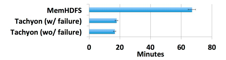
Performance comparison for realistic workflow. The workflow ran 4x faster on Tachyon than on MemHDFS. In case of node failure, applications in Tachyon still finishes 3.8x faster.
