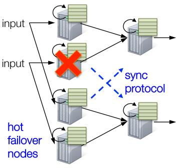
Separate set of "hot failover" nodes process the same data streams
