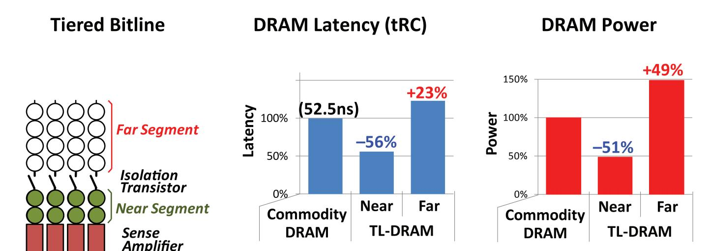
Area cost: 3% (due to isolation transistor)
