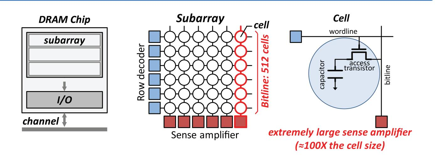
Long Bitline: Amortizes sense amplifier's overhead → Small area Long Bitline: Large bitline capacitance → High latency
