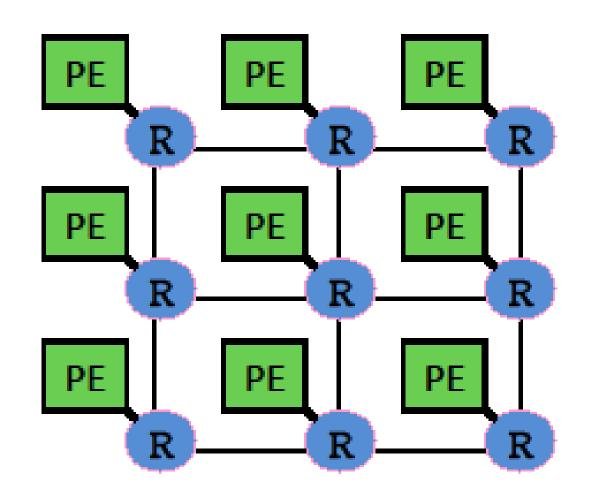
Network has limited shared resources (buffers and links) due to on-chip design constraints (power, die size, wiring)
