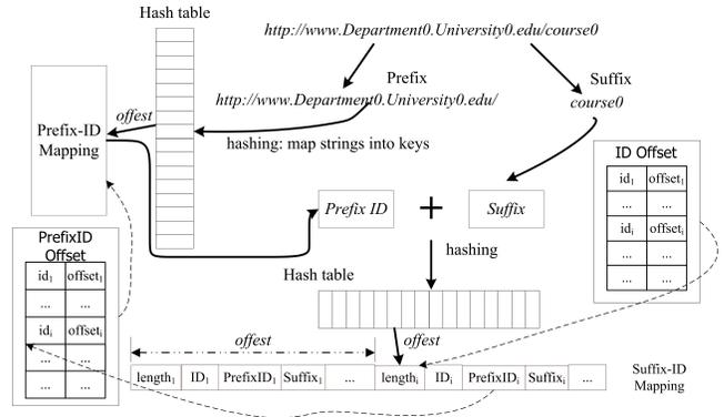
**Figure 1: String-ID Mapping and ID-String Mapping**
