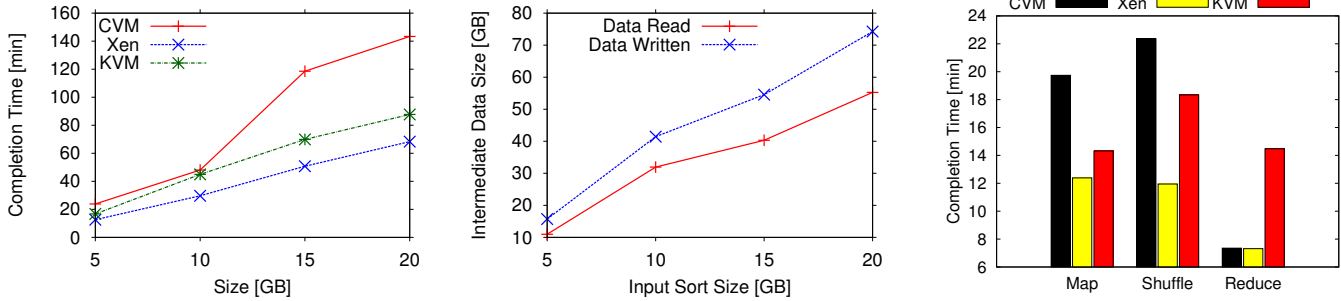
(a) TeraSort Completion Times. CVM has the longest completion time while Xen has the shortest completion time. As data size increases, CVM degrades the most compared to the other two hypervisors. (b) TeraSort Total Amount of Data Read and Written. The amount of intermediate data generated that is being written and read is significantly greater than the original sort size. This intermediate data degrades CVM's performance the most in TeraSort. (c) 10GB TeraSort Duration of Each Phase. CVM spends most of the time in the map (heavy in disk reads) and shuffle (heavy in both disk reads and writes). KVM spends a lot of the time during shuffle and reduce (heavy in disk writes).
